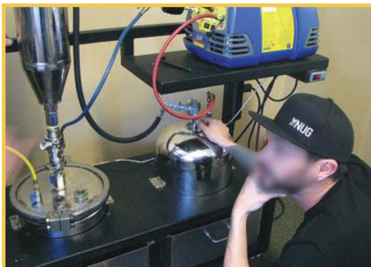
Counter clockwise from bottom right: butane reservoir, Yellow Jacket pump, packed cylinder, viewing port, BHO collection reservoir.
