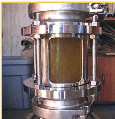
Closed-loop systems prevent you from seeing what's going on inside, save for the viewing vessel.
